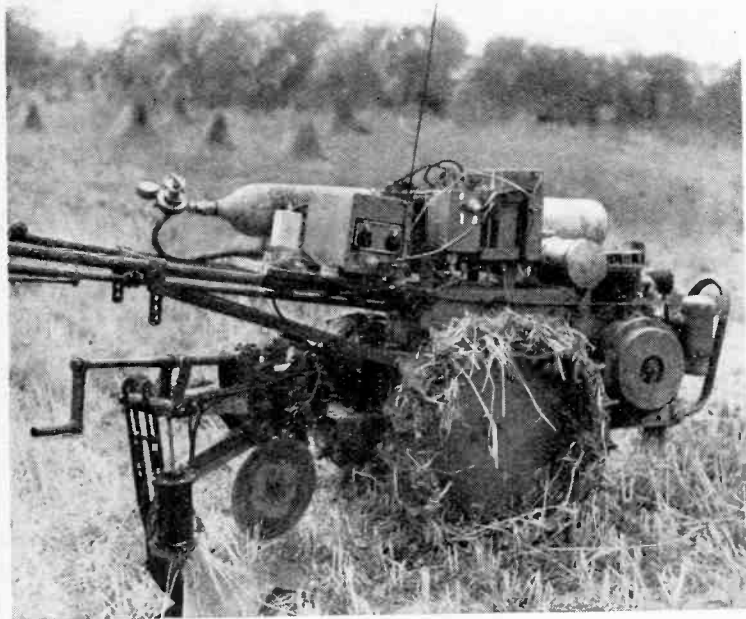
Radio equipment and automatic control gear mounted on the plough for the tests mentioned above. ("The Farmer & Stock-Breeder" photograph.)
